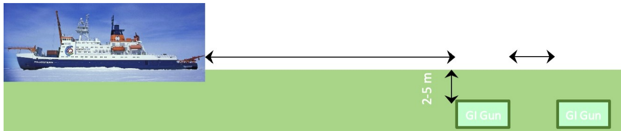
Figure A. 3: Sketch of Airgun array geometry (2 airguns), applied during Polarstern voyage "PS104" in February and March 2017 in Antarctica (dimensions not to scale).
