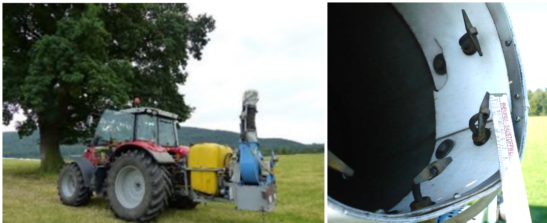
Figure 1: Tractor-mounted cannon sprayer KWH B 612 (left) with pneumatic atomiser (right).
