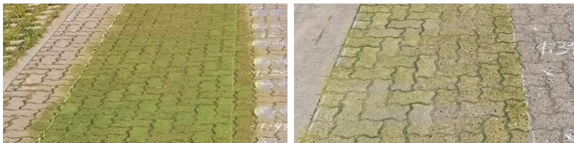
Figure 59: Trial area "paved path" after application with a knapsack sprayer and a brass nozzle (left) and an IDK 90-015 C nozzle (right).
