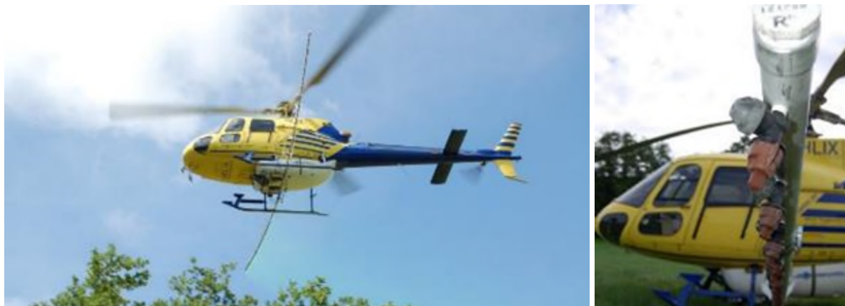
Figure 3: Eurocopter AS350 "Ecureuil" (left) with attached simplex spraying system (right).
