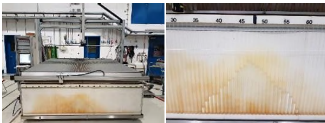
Figure 17: Single nozzle test bench for measuring the distribution accuracy of nozzles (left) and spray pattern in the plastic cylinders (right).
