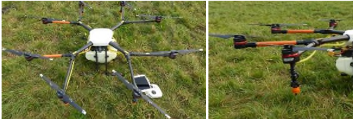
Figure 4: UAV Agras MG-1 from DJI (left) with attached spray system (right).
