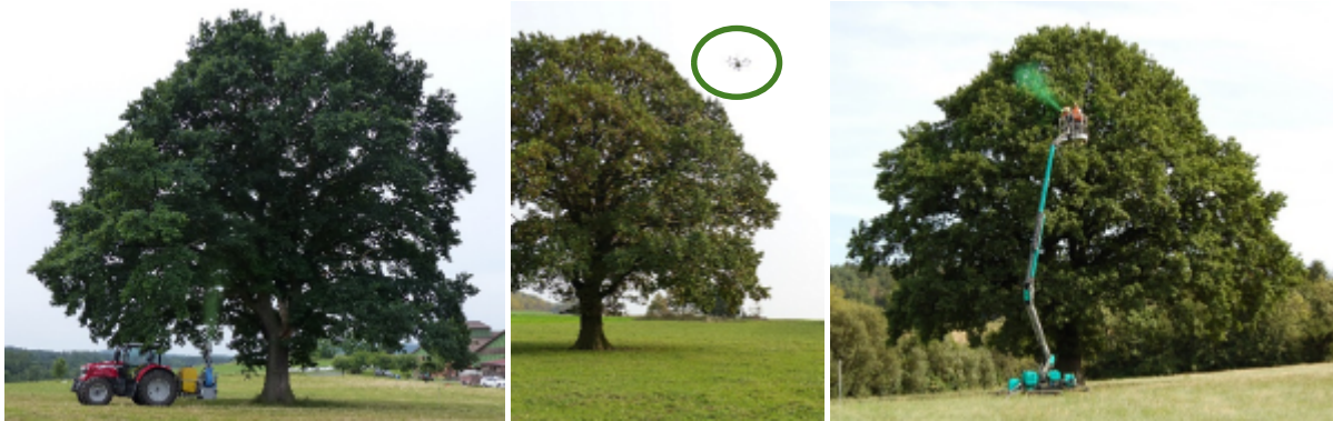
Figure 7: Use of a cannon sprayer with pneumatic atomisation (left), a UAV (centre) and a motorised knapsack mistblower (right) on the trial area “solitary tree”.
