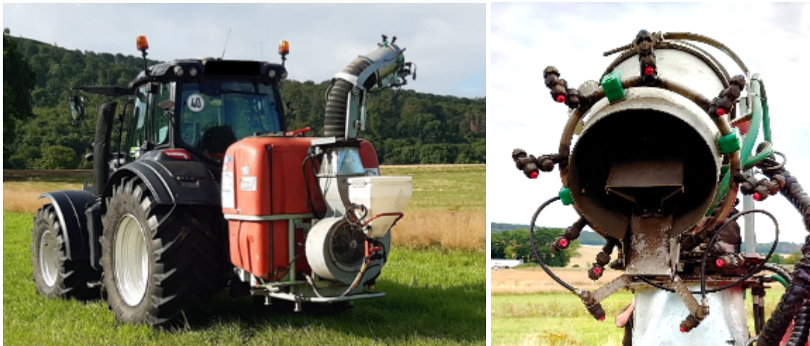
Figure 2: Tractor-mounted cannon sprayer Dragone AZ2 (left) with hydraulic atomiser (right).
