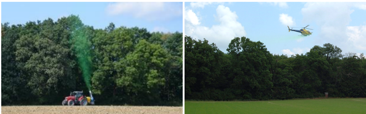
Figure 11: Use of a cannon sprayer with pneumatic atomisation (left) and a helicopter (right) on the trial area “forest edge”.
