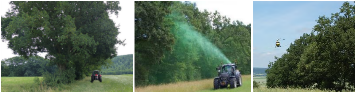
Figure 9: Use of a cannon sprayer with pneumatic atomisation (left), a cannon sprayer with hydraulic atomisation (centre) and a helicopter (right) on the trial area "avenue".
