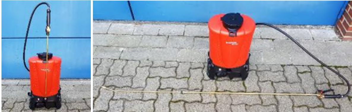
Figure 6: Knapsack sprayer with a normal lance (left) and long lance (right).
