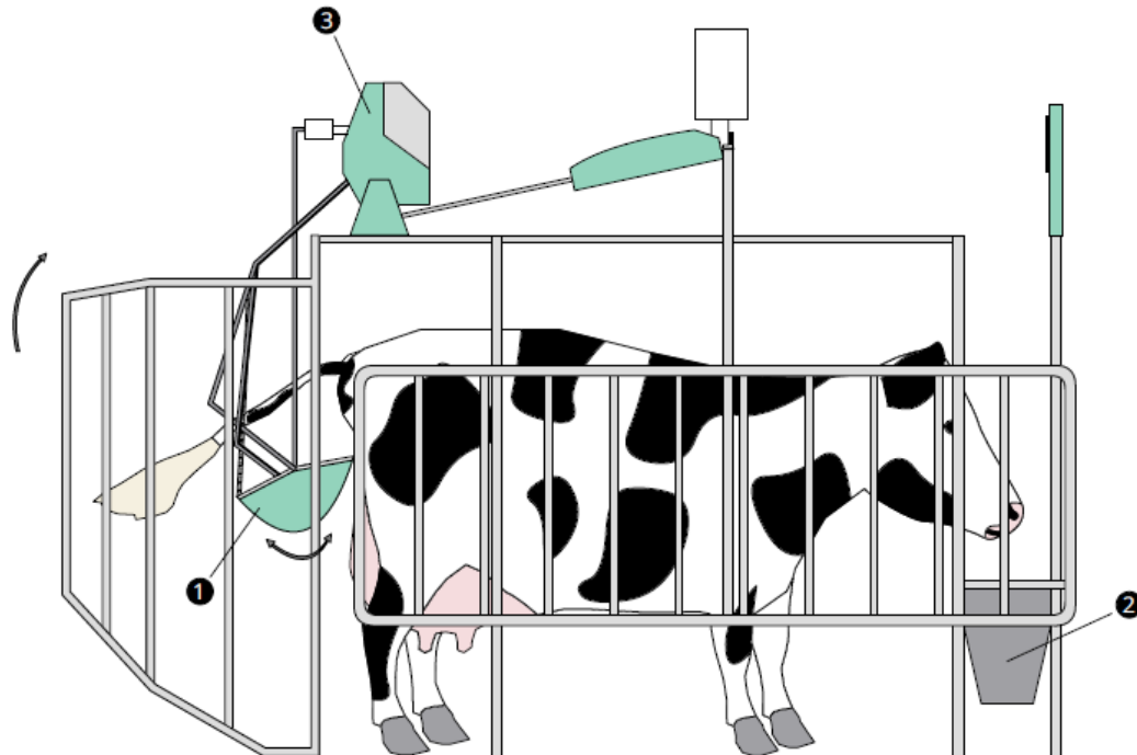
Figure 46: Sketch of a urine catchment and collection device
