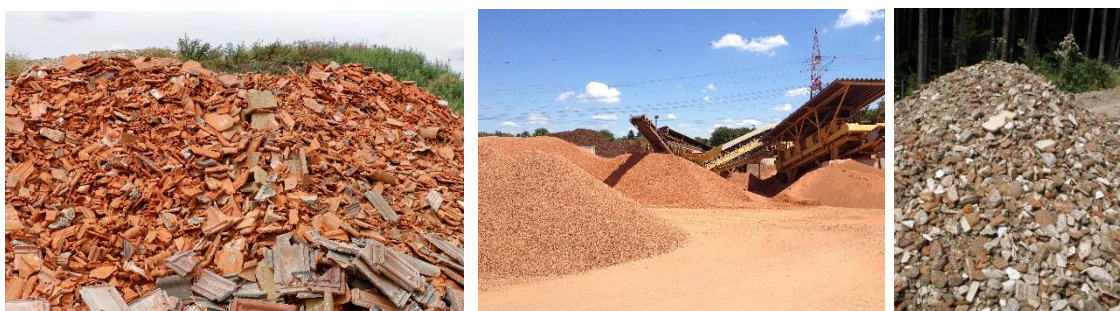
Picture 3: Used roof tiles separated for recycling (le.), chippings won from used bricks and roof tiles (ce.) and brick-containing recycled aggregate for a road base (ri.)
