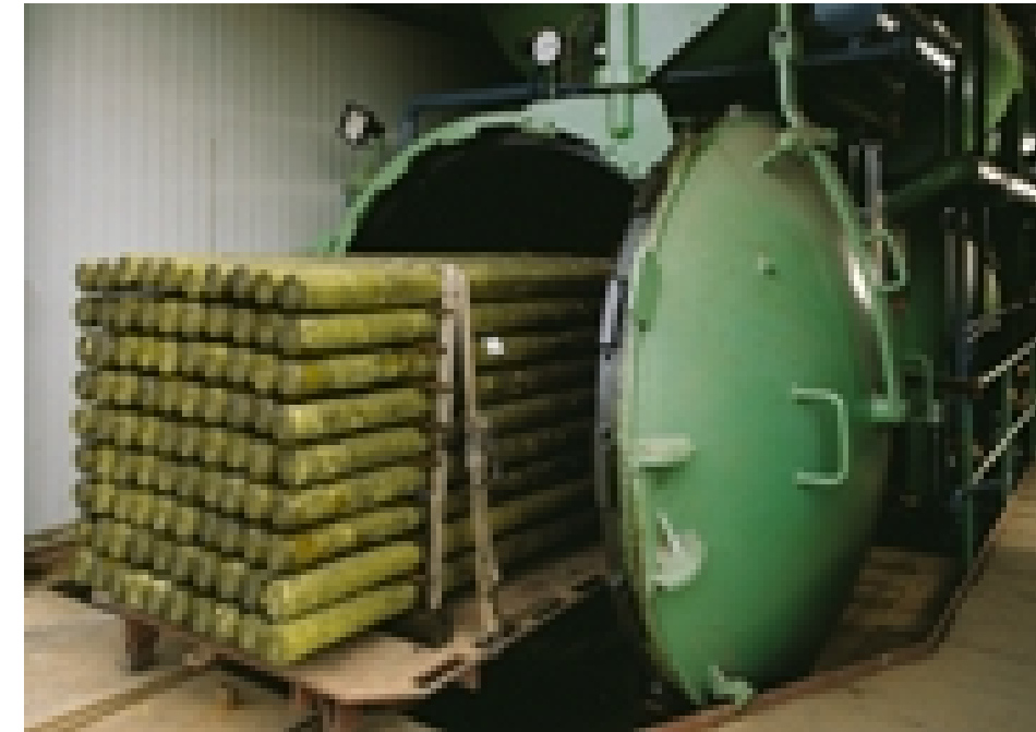
Vacuum-pressure impregnation for use class 3 and class 4 treated wood
